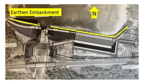
B) The Auxiliary Spillway is new to Secord Dam. It is designed to safely manage overflow. This concrete structure will be about the size of a football field and will have stair steps to help reduce the velocity of water should it flow over the Auxiliary Spillway. It will also include what Mike calls a "Toboggan Run" to disperse the overflow water into the river below the dam. This is a significant engineering / construction project.
