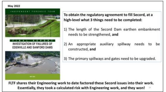
Using drawings of the dam, Mike explained in simple terms the work that is underway to meet the <u>requirements</u> established by EGLE. These key points are identified by the corresponding drawing below.
